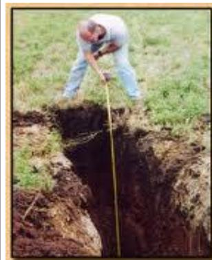
**3rd Test** The [Percolation Tests](#). If the water soaks away either too fast or too slowly, then a soakaway drainage field is not permitted. In general, clay soils will fail and it is not worth performing the tests. This is the test that most people associate with soakaway tests, as it has been mandatory for much longer than the TSAH. The Percolation Test tests the porosity of the soil immediately below and surrounding the 300mm. of drainage stone in the trench below the pipe.
