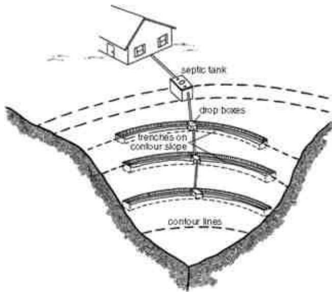
A foul water soakaway drainfield is NOT a 'Pit filled with stones' or 'Crates' etc. These types of sewage effluent soakaways are built by 'Cowboys' who don't know the regulations. They are ONLY allowed for surface roof water, NOT sewage effluent.
